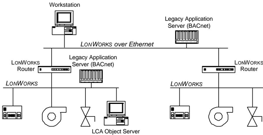
Figure 4. A fully distributed LONWORKS system with an Ethernet backbone using BACnet Servers
