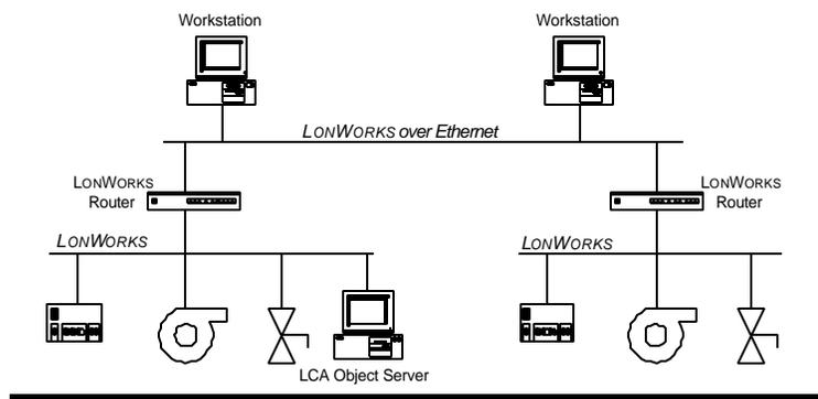
Figure 3. A fully distributed LONWORKS system using an Ethernet backbone
